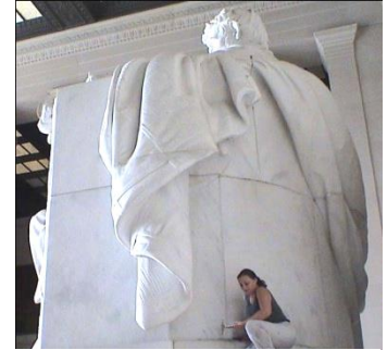
Sampling mortar at the Lincoln Memorial Washington, DC
