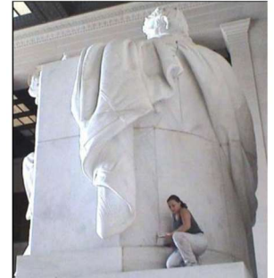
Sampling mortar at the Lincoln Memorial, Washington, DC
